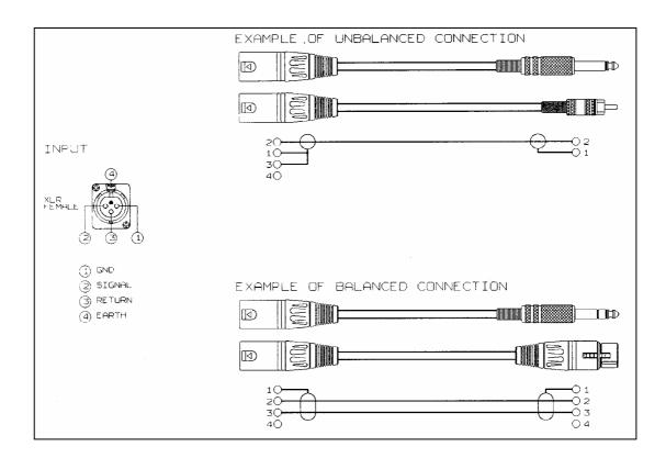
NOTE: The SEND female, 3-pin XLR input receives audio from microphone or mixer. If using a single microphone that needs phantom power to operate, you must supply this power to the microphone. The digital hybrid does not supply phantom power. Line/Mic input level selection is done through front panel DIP switch # 4.
