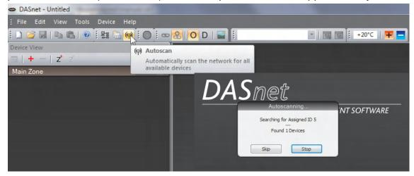
When the scanning process ends, all connected devices (on line) appear on the *device view window* in green.
