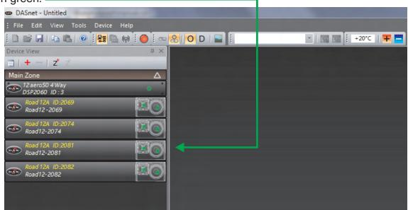
Important: only connected devices will appear on the main window. If the communication with any of the devices is lost after being detected, the unit will appear in red colour and physically in the cabinet the Comms / ID led will not light up:
