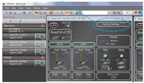
But also physically by pressing the preset knob (holding during a few seconds) while powering the cabinet (on the Road 12A / 15A and LX-218CA).
