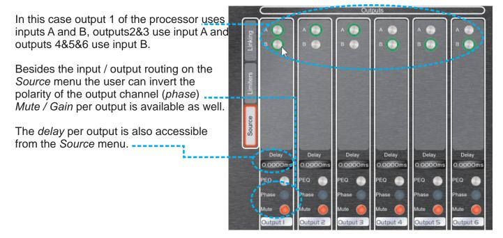
On the *Linking* menu the user can link channels. When two channels are linked all parametres are copied on both channels; gain, Eqs., delay, Xovers. Warning: polarity doesn't link between
