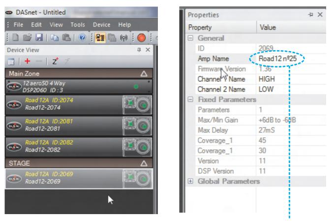
The ID number on the cabinets is unique and will never change. The user can rename the cabinets by using an easier code, for instance numbers: Road 12 nº25 etc
