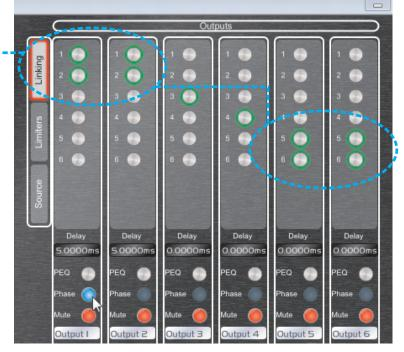
On the *Limiters* menu the user can set up the limiter threshold, attack and release time per output. There are two ways of working with the limiters, *automatic (auto ON)* mode which uses the Xover frequencies on each output to calculate the time constants. The user only sets the threshold. Or *manual (auto OFF)* mode; in this case the user defines the attack and release times.
