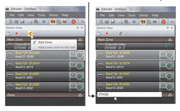
The unit Road 12A ID:2069 has been moved to the Zone named STAGE. Besides this, the unit could be renamed on the properties window (this name will remain in the memory of the device!):
