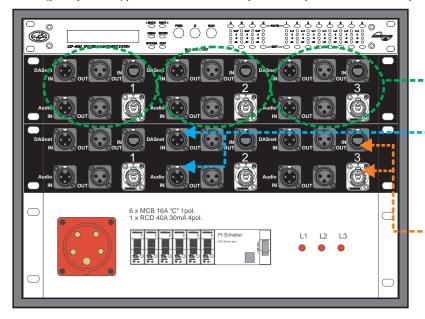
The patch panel has different "zones" limited by the maximum current allowed by the powerCon conector (20A).
