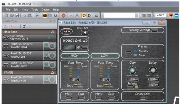
When it is switched off all values are saved in the internal micro controller memory, so next time the system is powered the parameters remain the same Gain +3dB, delay 5.033ms.
