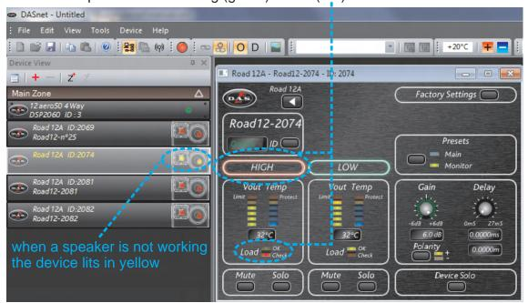
On the "advanced view" parameters as gain/delay/preset/polarity/mute and solo are available:
