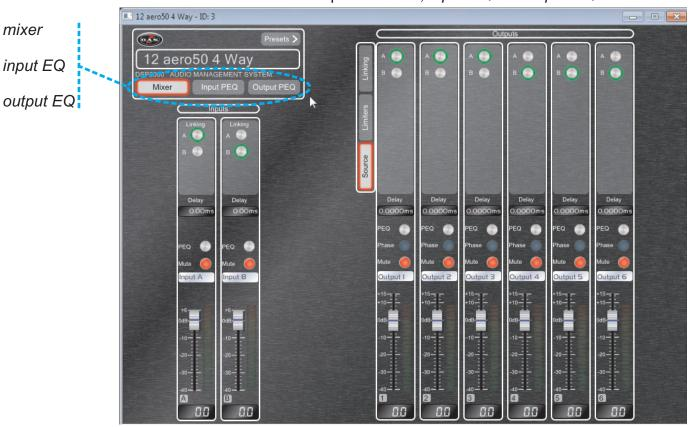
On the *Mixer* menu three options are available: *Source*, *limiters* and *Linking*. *Source* is the input matrix and can be used for routing inputs and outputs.
