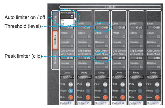
Threshold level will set up the RMS limiter value and Clip Level Above will set up the Peak limiter.
