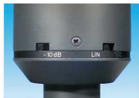
The -10 dB function is achieved by reducing the capsule polarizing voltage from 60 V to 23 V. It helps to avoid overloading the following units during very high sound pressure levels.
