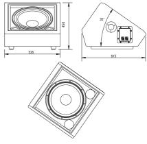
and a compression driver mounted coaxially. handled by a 1" exit compression driver with 1.75" titanium diaphragm and voice coil,
