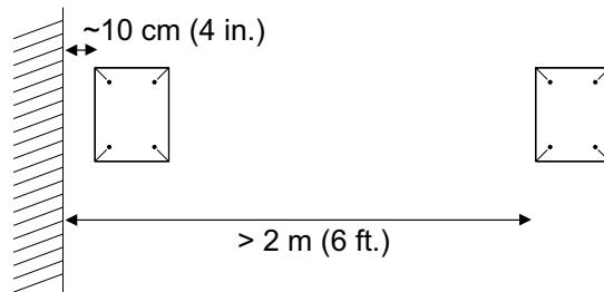
Placing the speaker in the middle of a room (i.e. not against a wall) will require +3 dB low frequency equalisation.
