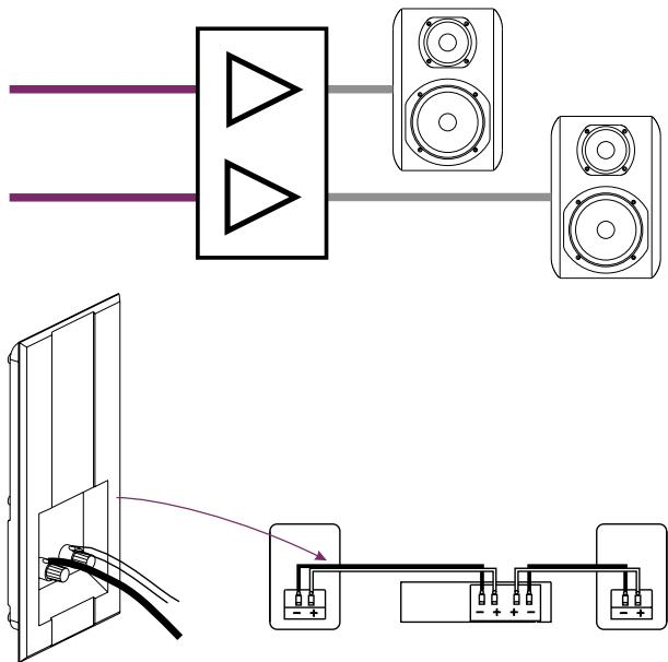
An amplifier for a MONITOR 6 should have an RMS power output between 100 W and 200 W at 8 ohms. An amplifier for a MONITOR 6 should have an RMS power output between 125 W and 250 W at 8 ohms. Use the largest amplifier you can within the recommended power range.
