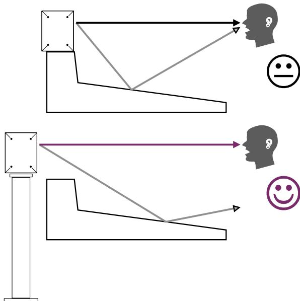
The MONITOR series can be used both in either horizontal or vertical orientation, although the latter is recommended.
