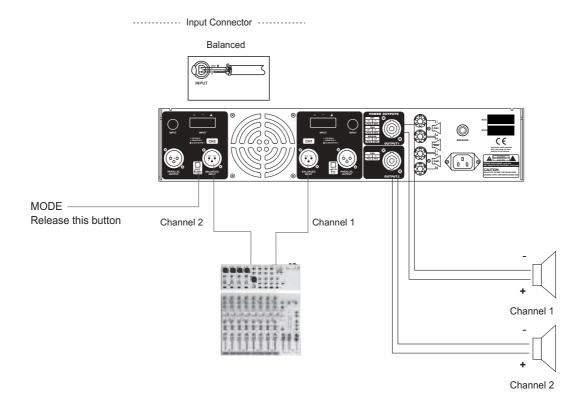
You can also operate the paralleled mode via outside wiring, so, the signal input from channel 1 or 2 will be output from both channel 1 and 2 simultaneously. The volume of channel 1 or channel 2 can be controlled separately.
