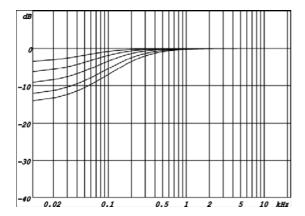
Hi EQ: can be set from +1 to -4 dB (in 1 dB increments), as shown in the diagram below:
