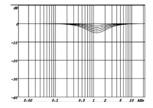
Bass EQ: can be set from 0 to -10 dB (in 2 dB increments), as shown in the diagram below, without effecting the Low Cut frequency setting.
