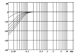
• **Mid EQ:** can be set from 0 to -5 dB (in 1 dB increments), as shown in the diagram below:
