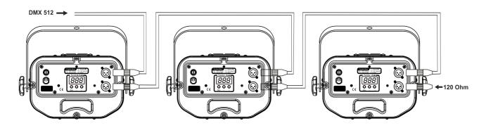
The wires must not come into contact with each other, otherwise the fixtures will not work at all, or will not work properly.
