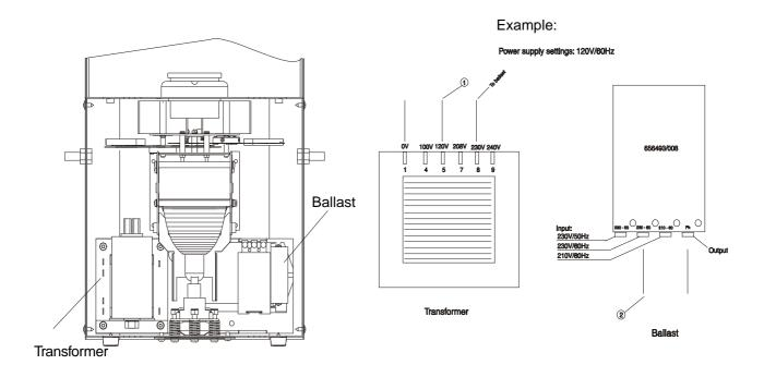
4. Put the cover back before applying AC power.
