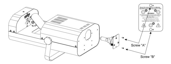
To insert the lamp open the small cover at the rear panel (see the drawing) by loosening the 2 Phillips screws "A" and "B" on the cover.
