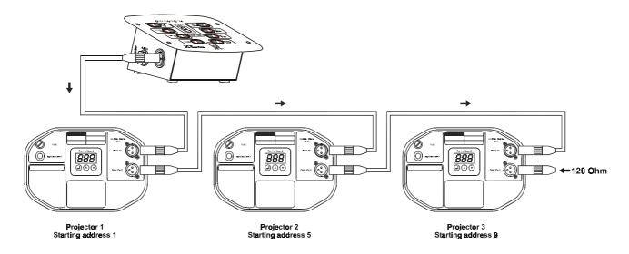
Only use a stereo shielded cable and 3-pin XLR-plugs and connectors in order to connect the controller with the fixture or one fixture with another.
