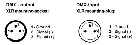
If you are using the standard controllers, you can connect the DMX-output of the controller directly with the DMX-input of the first fixture in the DMX-chain. If you wish to connect DMX-controllers with other DMX-outputs, you need to use adapter-cables.
