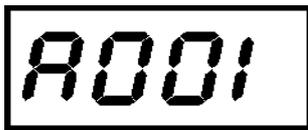
By this menu you can set the DMX address or address the fixture as a master/slave.
