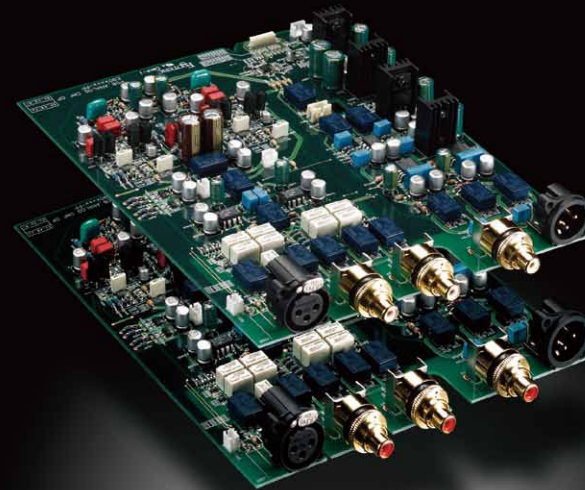
Fully balanced, dual mono audio boards
