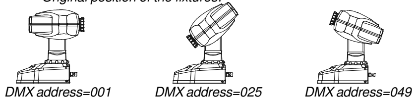
Tilt position is adjusted with the TILT wheel :
