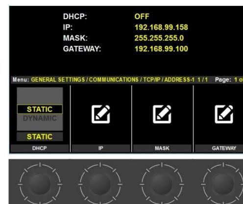
By rotating the 4 encoders you can set for a new IP Address.
