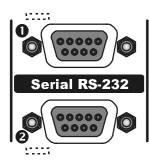
**RS-232 Serial port 1** features the Tx and Rx signals plus the DSR and CTS signals, and it is **dedicated** only to local, bidirectional connection whit an external computer running the Software Remote Control. Connect a standard serial cable (not crossed cable) between the RS-232 connector and a serial port connector on the computer. Typically, a DB-9 male to DB-9 female serial cable is required. Supported max Baud Rate: 19200.
