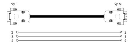
SERIAL **PORT 2** connection pin-out
