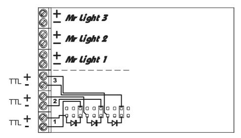
Mr Light LED lamps can be driven by external TTL tensions (+ 5 Volts) applied to terminal blocks from 1 to 3.
