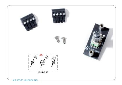
Position the drilling jig on an appropriate box and make the three holes. Install your cap in a box for switches and insert the PCB with the potentiometer coming out from the center hole. Secure with the two included screws. Cover the potentiometer with the gray knob.
