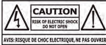
THE LIGHTNING FLASH WITH ARROWHEAD SYMBOL, WITHIN AN EQUILATERAL TRIANGLE, IS INTENDED TO ALERT THE USER TO THE PRESENCE OF UNINSULATED "DANGEROUS VOLTAGE" WITHIN THE PRODUCT ENCLOSURE THAT MAY BE OF A SUFFICIENT MAGNITUDE TO CONSTITUTE A RISK OF ELECTRIC SHOCK TO PERSONS.
