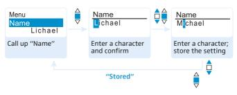
Via the "Name" menu, you can enter a freely selectable name (e.g. the name of the performer) for the radio microphone.
