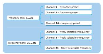
Each of the channels in the frequency banks "1" to "20" has been factory-preset to a fixed transmission frequency (frequency preset).
