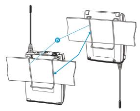
The belt clip is detachable so that you can also attach the transmitter with the antenna pointing downwards. To do so, withdraw the belt clip 19 from its fixing points and attach it the other way round.
