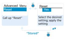
When resetting the bodypack transmitter, only the selected settings for the pilot tone and for the frequency banks "U1" to "U6" remain unchanged.
