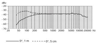
**Specifications** Transducer principle pre-polarized condenser microphone 20-20.000 Hz Frequency response half-cardioid Pick-up pattern Sensitivity 10 mV/Pa (free field, no load at 1 kHz) Nominal impedance (at 1 kHz)  $< 100 \Omega$ Min. terminating impedance 1 kO Phantom powering 48 V / 1.1 mA Max. sound pressure level at 1 kHz 136 dB SPL Connector XI R-3 Weight 350 q Dimensions Length: 126.5 mm Width: 105 mm Height: 26.5 mm
