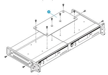
Secure the jointing plate 22 to the receivers using six recessed head screws (M 3x6).
