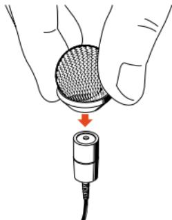
Please install the MZW 2 wind-shield, first. This wind-shield reduces the wind noise by a maximum of 20 dB.
