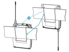
The belt clip is detachable so that you can also attach the transmitter with the antenna pointing downwards. To do so, withdraw the belt clip (B) from its fixing points and attach it the other way round.
