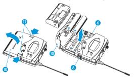
Insert the two batteries or the accupack as shown above. Please observe correct polarity when inserting the batteries/accupack.
